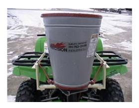
Designed to save time when you need to spread in less then favorable weather conditions. The Precision ATV seeder mounts on most all terrain vehicles for spreading seeds, fertilizer, granular insecticide and herbicides.
