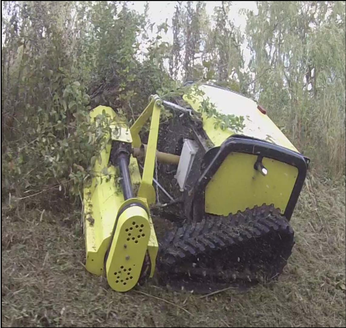
The Danish-produced special lawnmower Lynex TX1100, with its simple construction and low center of gravity, works on slopes up to 60 degrees.
